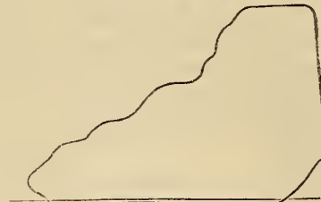
B. High-pressure—Top of Cylinder. Steam in Boiler ..... 115 Vacuum ..... 18 Revolutions ..... 52
